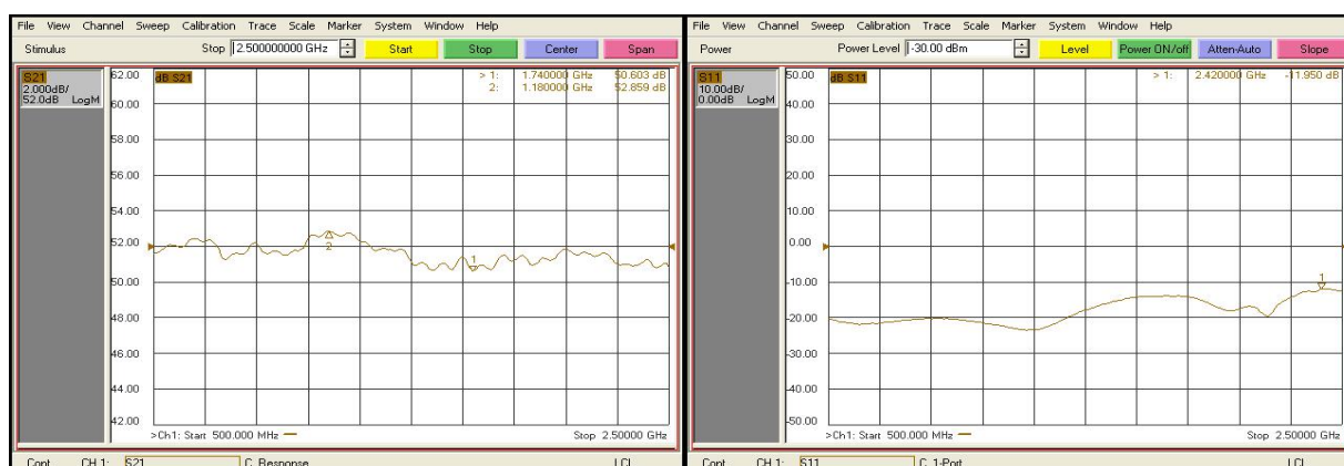
Figure left: Power Gain S21 (Pin=0dBm, Load VSWR≤1.2, 25°C), For reference only.
