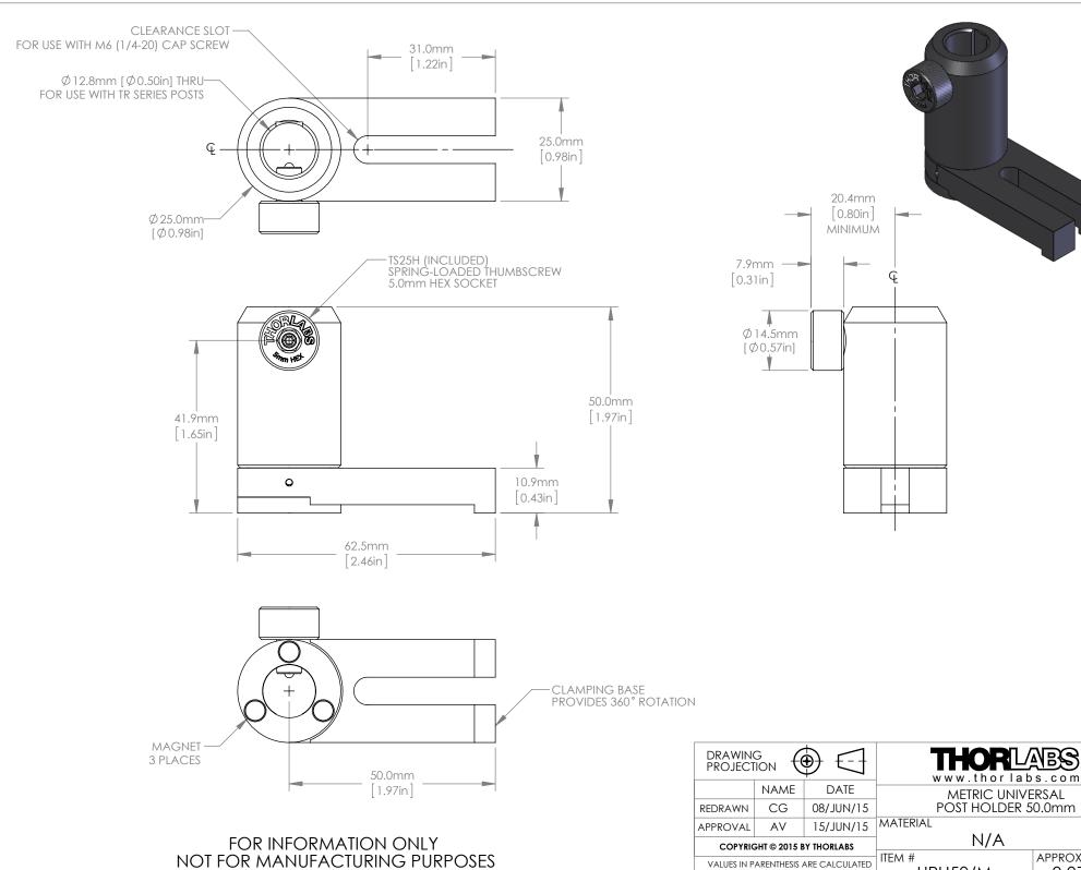
METRIC UNIVERSAL POST HOLDER 50.0mm REV COPYRIGHT © 2015 BY THORLABS APPROX WEIGHT ITEM # VALUES IN PARENTHESIS ARE CALCULATED UPH50/M 0.07 kg AND MAY CONTAIN ROUNDOFF ERRORS
