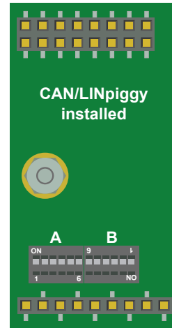
Setting of DIP switches A: all ,on' / B: all ,off'
